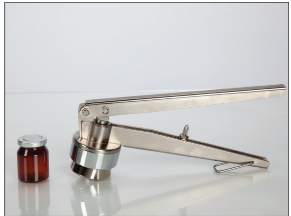
Step 2. After placing the cap on the vial, place the mouth of the crimper onto the cap.
