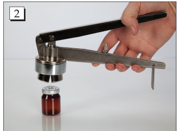
Step 2. After placing the cap on the vial, place the mouth of the crimper onto the cap.
